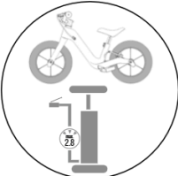
The tires are not fully inflated during transport. It is necessary to inflate the tires to max. 2.8 bar before first use.
