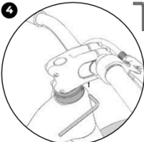
Adjusting the handlebars: The handlebar height can be adjusted extensively, allowing the balance bike to grow with the child (see recommendations for setup on p. 106). To adjust the handlebar height, first loosen the shaft clamp (1) under the stem with a 5 mm Allen key.
